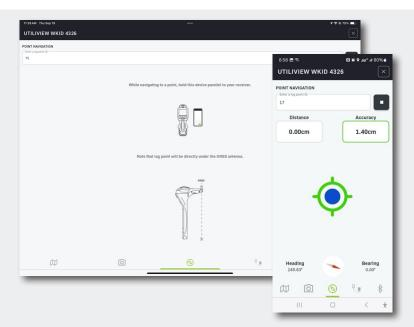
Use Subsite<sup>®</sup> Point Navigation to effortlessly return to unlimited previously located points, reducing guesswork and improving field efficiency.
