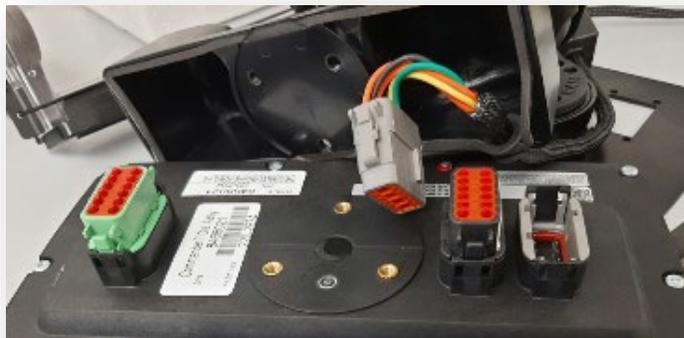
d) Plug 222-2661 field update harness into display and connect to CAN bridge harness (in dash connector).
