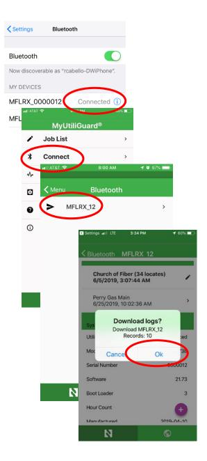
Bluetooth connect the mobile device to the receiver. Open the MyUtiliGuard app and download the log.
