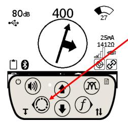
The user must press and hold the depth button to record a log point.
