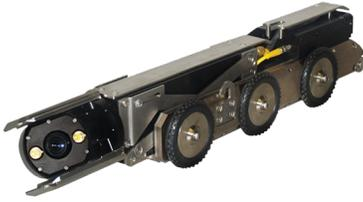
**Contractor-grade mainline inspection system for 6- to 30-inch diameter pipes and pipe runs up to 2,000 feet.**
