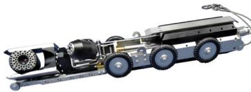
**Inspect mainlines 6 to 24 inches and laterals 4 to 8 inches in diameter simultaneously.**
