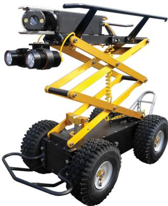
**Steerable four-wheel-drive transporter for inspecting storm drains, sewer, and water pipes 24 inches and larger.**
